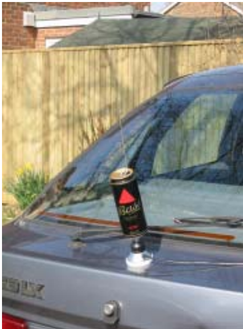
The new 2m quarter wave antenna
